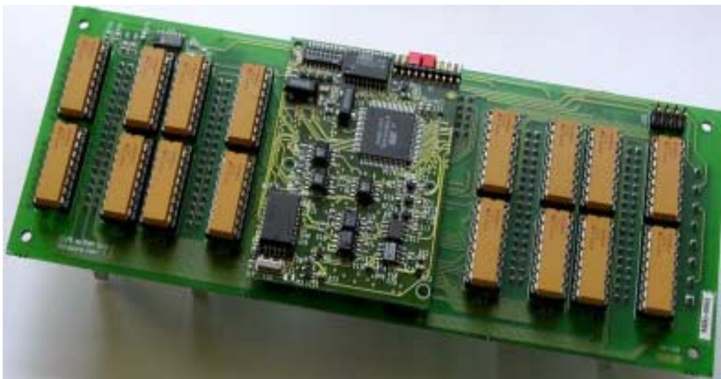
Figure 3.7: Back side of the mother board with the ELMB and 16 signal adapters for analogue inputs.
