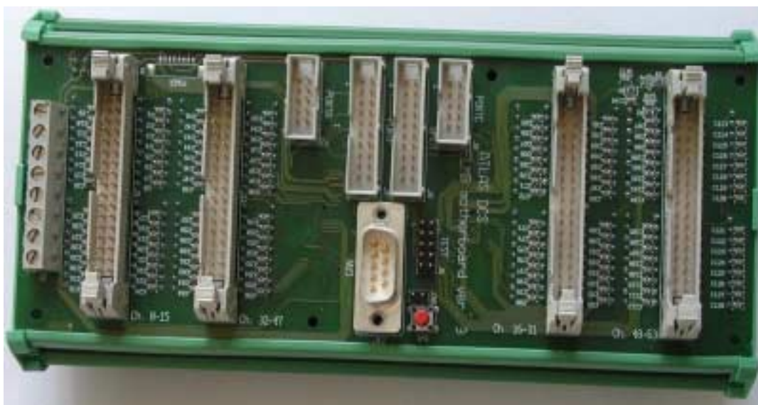
Figure 3.8: Front side of the ELMB mother board with 4 connectors for analogue inputs, digital ports A, C and F, SPI bus, power connector and CAN bus connector.
