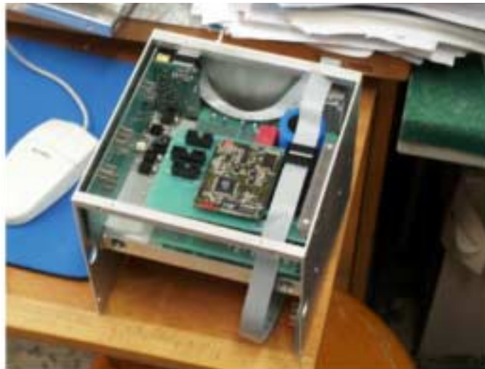
Figure 6.6: ELMB embedded in the electronics of the finger LV power supply.
