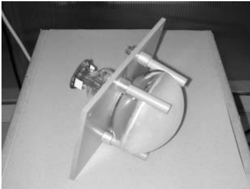
Figure 6.45: PMT final assembling. The TPB coating on the PMT glass window is clearly seen. The voltage divider has been mounted directly on the PMT output leads.
