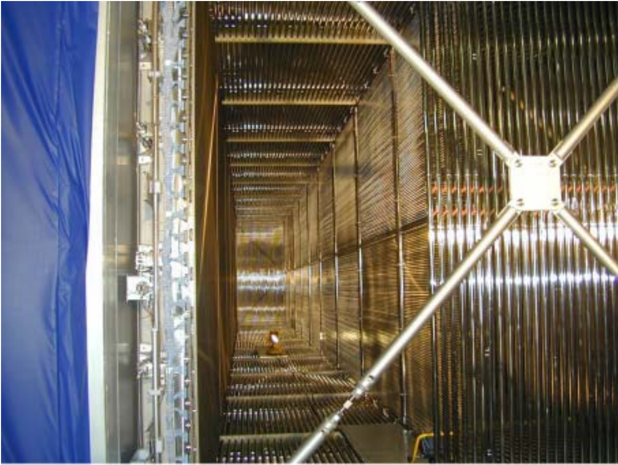
Figure 6.20: Photograph of the internal detector assembly in the T600 first half-module. Central cathode and race-tracks may be clearly identified.
