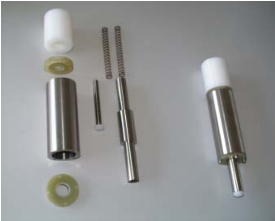
Figure 6.25: Picture of a wall position meter. On the left side the sensor is decomposed in its parts, and on the right side it is assembled.
