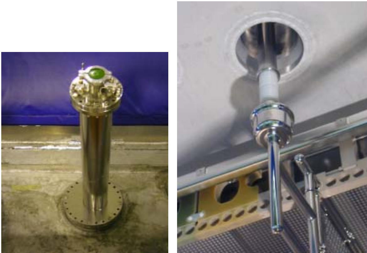
Figure 6.34: Left: the HV feedthrough positioned on the T600 roof flange. Right: details of elastic contact between the feedthrough and the receptacle connected to the cathode.
