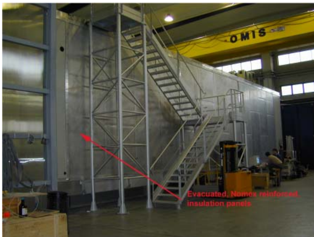
Figure 6.13: Photograph of the T600. The lateral wall insulated with evacuated Nomex panels is indicated.
