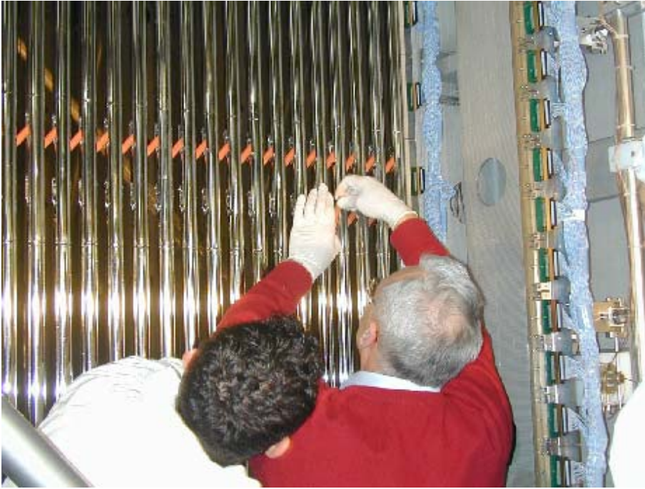
Figure 6.35: Installing the resistors for the HV divider.
