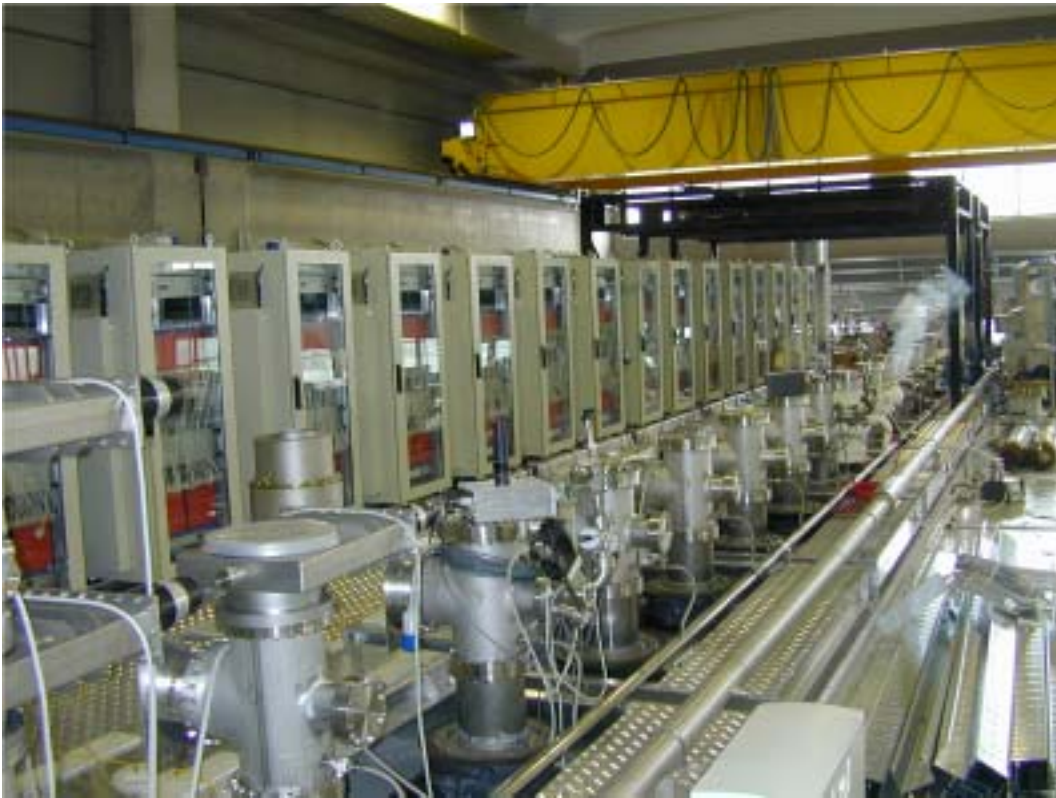
Figure 6.50: Photograph of the T600 top showing the disposition of the electronic Racks for one chamber.
