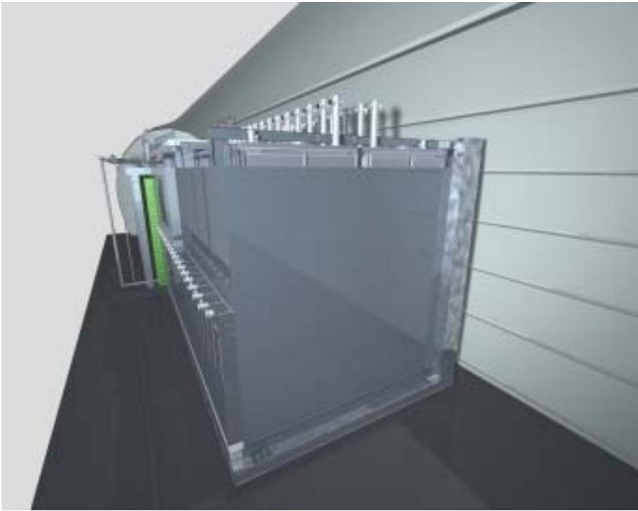
Figure 8.9: T1200 installation: assembly of the retaining tank and of the thermal insulation.
