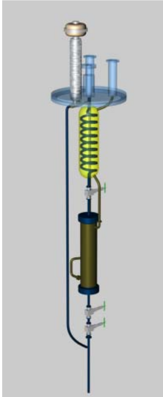
Figure 6.15: Drawing of the gas recirculation unit. The argon (blue piping for colour copies, yellow is for \text{LN}_2 distribution piping) is liquefied in the recondenser on the top and passes through the Oxysorb cartridge to be re-injected near to the surface of the liquid in the main container. The recondenser and the filter are sealed in a vacuum tight barrel (not shown in the drawing) for thermal isolation purposes.
