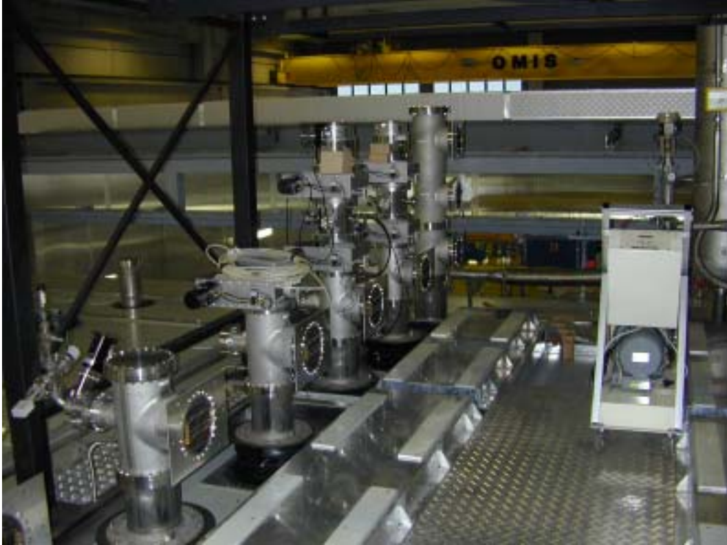
Figure 6.7: Picture of the T600 vacuum pumping units, on the top of the dewar.
