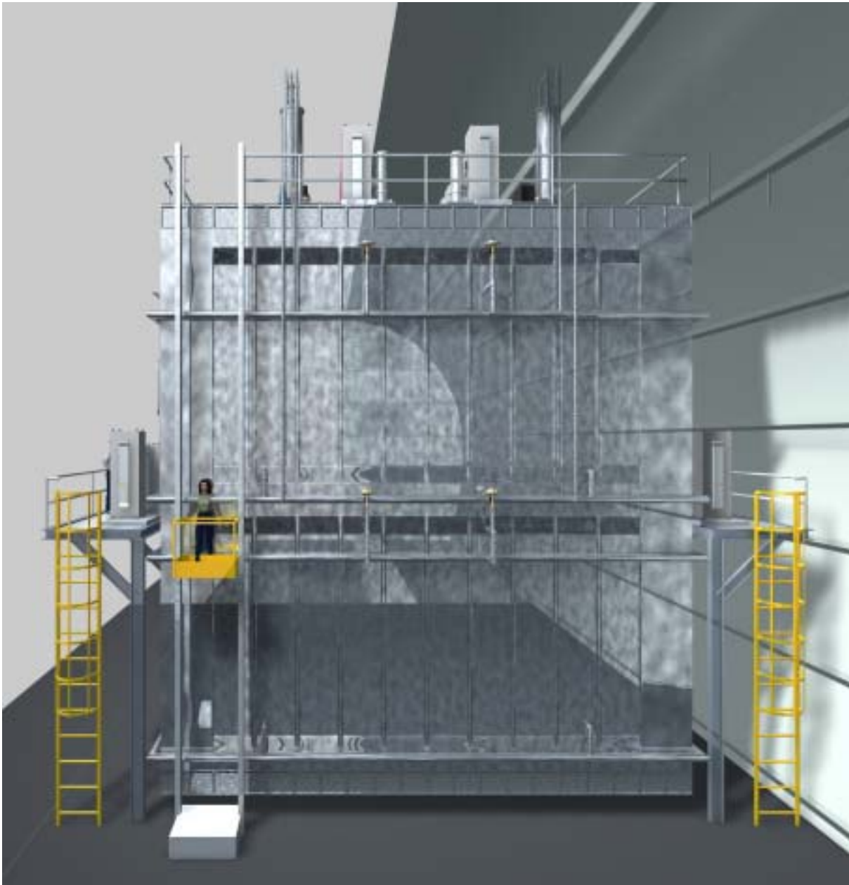
Figure 4.4: Front view of the ICARUS 2\times T1200+T600 detector as seen from a neutrino coming from CERN.
