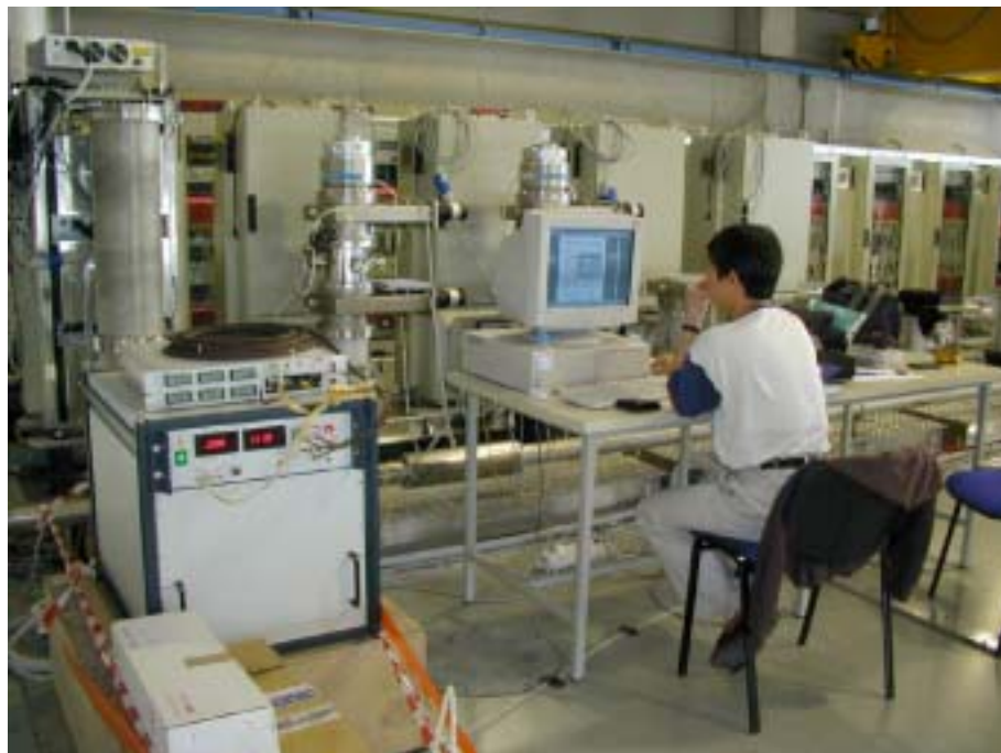
Figure 6.38: HV equipment on the top of the T600 detector (HV power supply, HV monitor, interface to Ethernet, remote control and monitoring software running on a PC).
