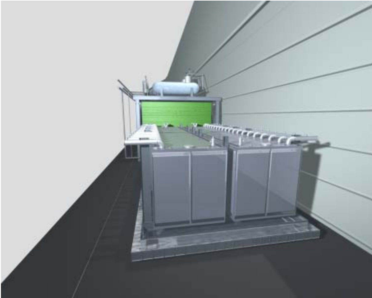
Figure 8.7: T1200 installation: lower two LAr containers.
