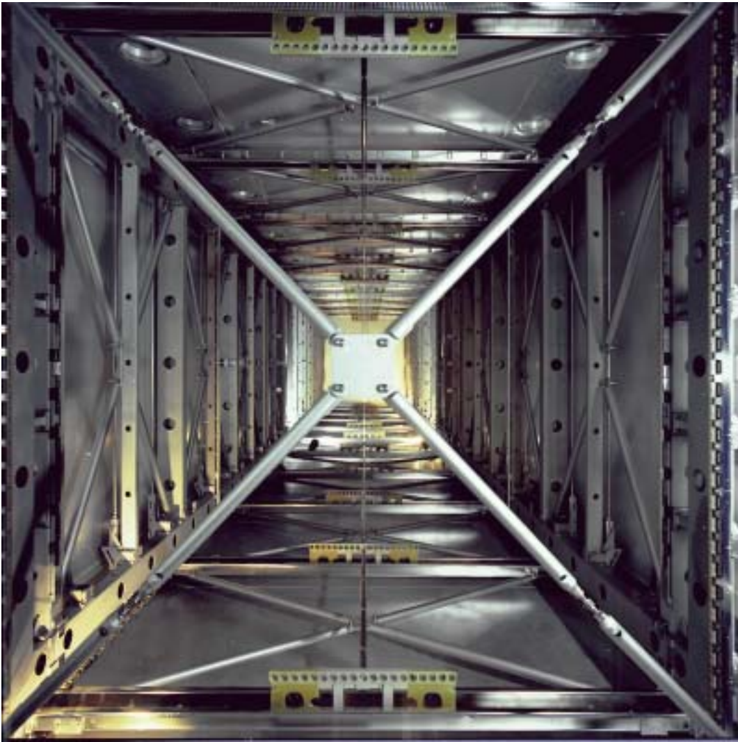
Figure 6.19: Photograph of the internal detector sustaining structure installed in the T600 first half-module.
