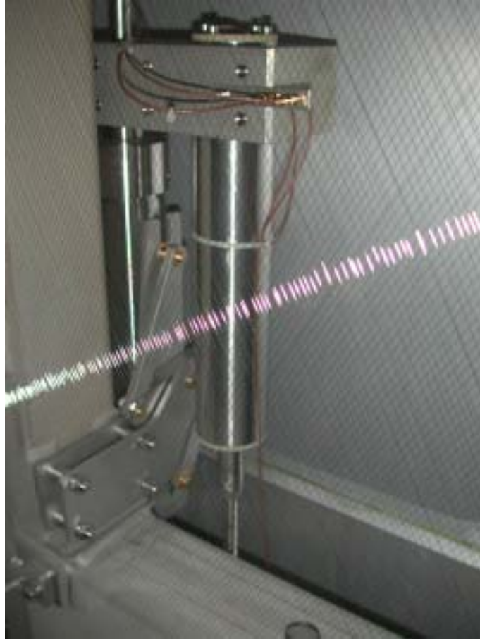
Figure 6.29: Position meter for vertical wires mounted behind the wire chamber.
