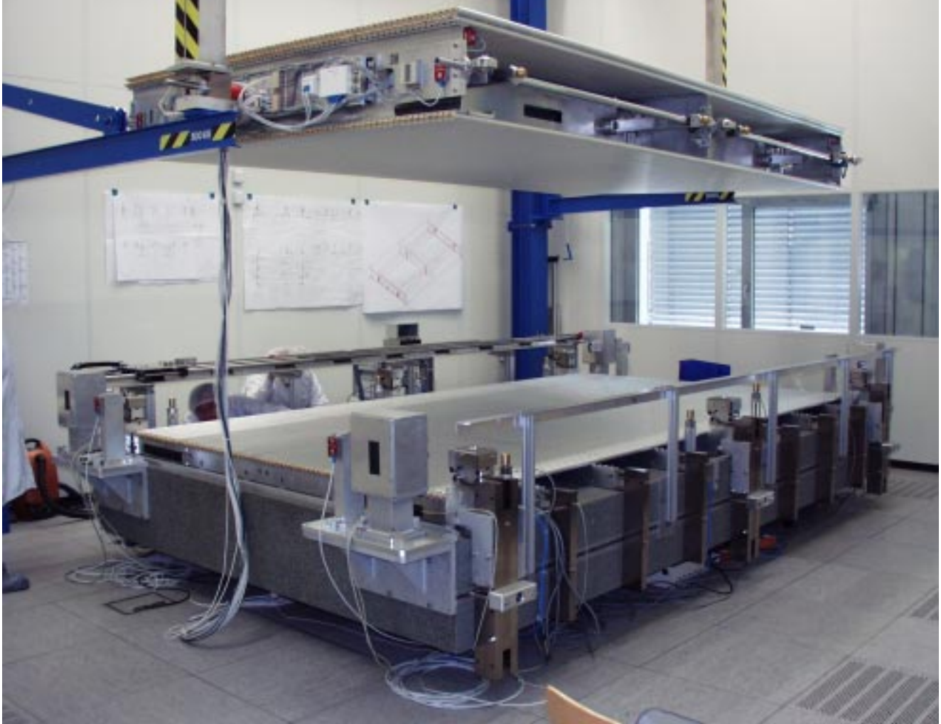
Fig. 3. Assembly facility for BOS MDT chambers with the first chamber under construction.
