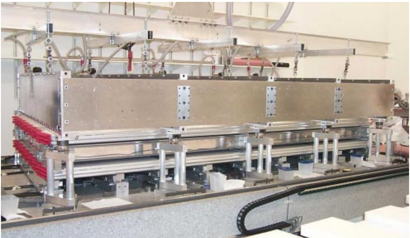
Fig. 4. Assembly table for endcap MDT chambers with the stiff auxiliary frame.
