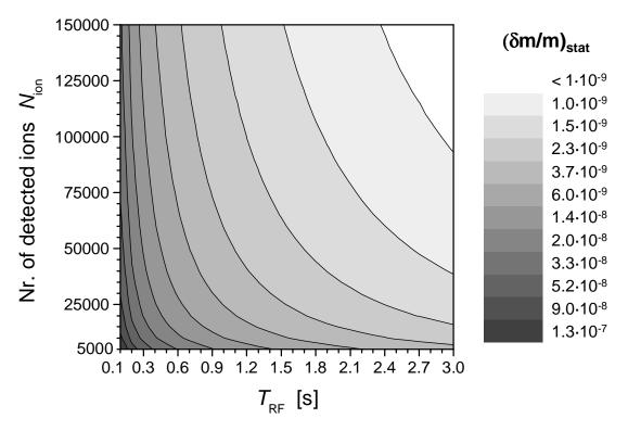
Figure 5: The statistical uncertainty ( $\delta m/m$ )<sub>stat</sub> as a function of the observation time  $T_{RF}$  and the number of detected ions  $N_{ion}$  for an ion with mass number A = 100 in a magnetic field of B = 6 T.
