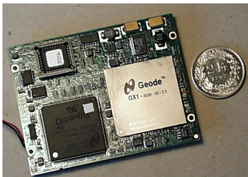
Figure 39 Photograph of a Credit-Card PC. A two-franc coin is shown for size comparison.
