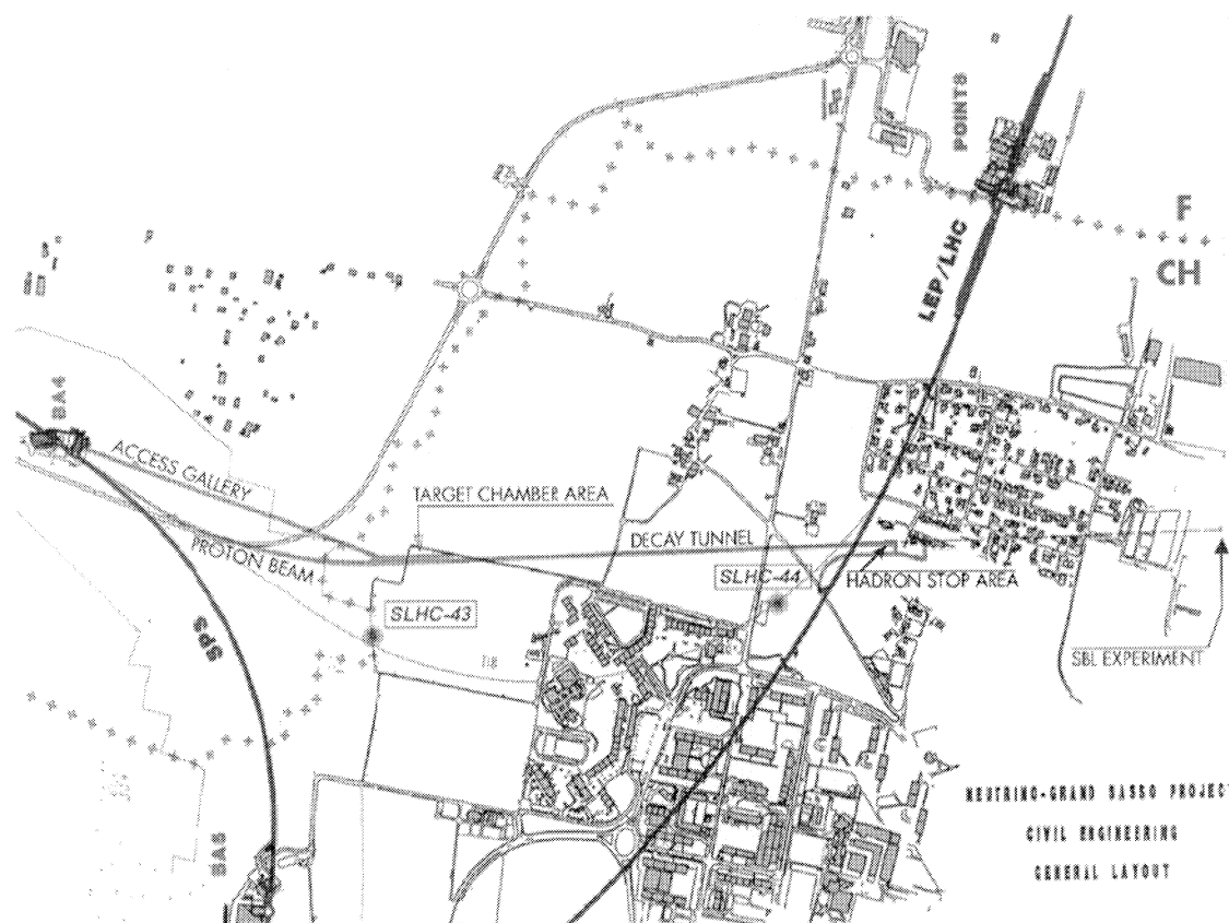
Figure 3.1: Layout of the NGS at and around CERN including the 2 positions of the drillings SLHC-43 and SLHC-44.
