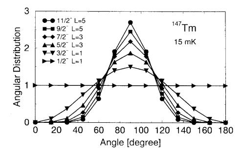
half life, forms just a multiplication factor in the experimental angular distribution. In this way, the L-value of the proton wave and the emitter spin, extracted from angular distribution, are model independent.
