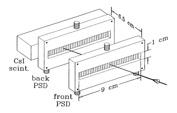
FIG. 2. Detail of a telescope, consisting of two Micron, Inc. Model TT position-sensitive detectors and a CsI(Tl) scintillator crystal; for more details see the text. An example ejectile track is shown.
