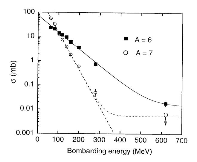
FIG. 8. Total cross sections for mass-6 and mass-7. The fits are described in the text (Eqs. 7-9).
