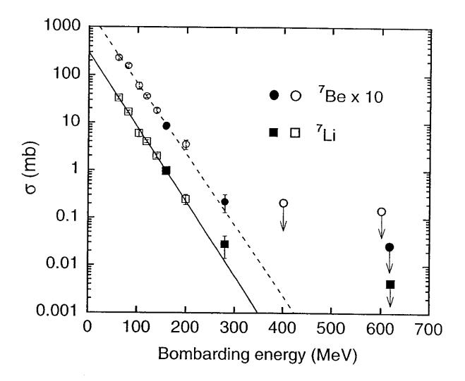
FIG. 7. Total cross sections for  ${}^{4}\text{He}(\alpha, n){}^{7}\text{Be}$  (circles) and  ${}^{4}\text{He}(\alpha, n){}^{7}\text{Li}$  (squares). All  ${}^{7}\text{Be}$  values are multiplied by 10 for clarity. Solid symbols are from the present experiment, and the open symbols are from previous work as summarized in Table II. The lines are exponential fits as described in the text (Eqs. 5, 6).
