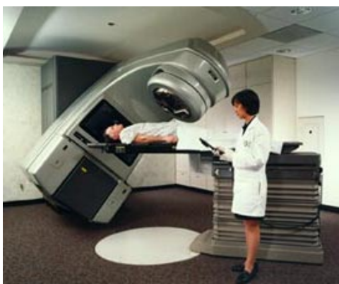
Figure 1-2: Example for a (photon) gantry that allows the irradiation from multiple entry ports. The electron linear accelerator is mounted directly in the head of the rotating machine. Source: Varian Medical Systems [online], available from: http://www.varian.com/prd/prd102.html , [accessed 5.5.2000].
