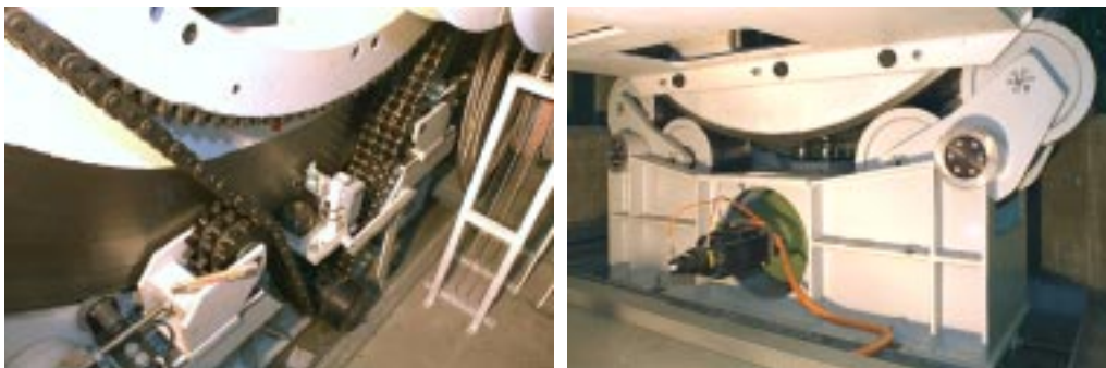
Figure 2-15: The rear ring of the PSI proton gantry showing its chain drive and the roller supports. Source: Schär Engineering AG
