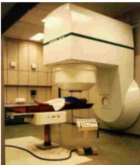
Figure 2-21: View (left) and section (right) of the isocentric neutron gantry installed at the NAC, South Africa. The neutrons are produced from a 66 MeV proton beam hitting a beryllium target. Source: The National Accelerator Centre (NAC), South Africa [on-line], available from: http://medrad.nac.ac.za/neuts.htm [accessed 2000-05-16]
