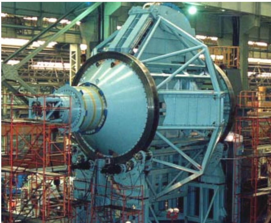
Figure 2-11: An isocentric proton gantry before installation in the NCC. Source: Ion Beam Applications (IBA).
