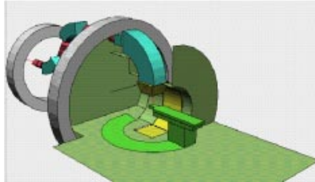
Figure 2-20: Proposed concept for a second, but this time isocentric, proton gantry at the PSI. The gantry turns only \pm 90^\circ , the patient couch performs a continuous 180^\circ rotation in the horizontal plane. Source: Pedroni, 2000
