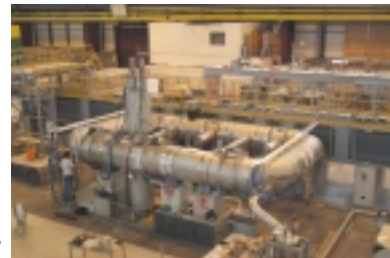
B0-coil connected to the test facility
