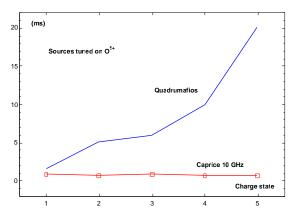
Figure 3: Confinement time of oxygen ions for two ion sources having different plasma volume
