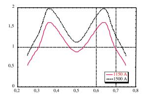
Figure 6: PHOENIX axial magnetic profils at 1150 A and 1500 A
