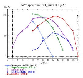
Figure 4: Ar spectrum for various ECRIS when they are tuned for 1 µAe on the maximum charge
