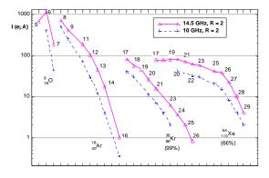
Figure 2: effect of the frequency on the performances of Caprice with R = 2 solid lines: 14.5 GHz, dashed lines: 10 GHz
