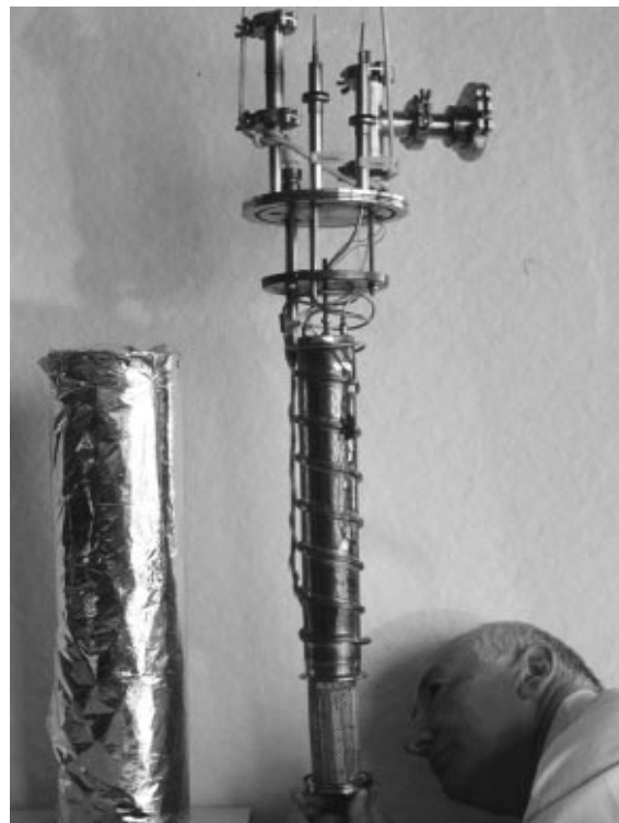
Figure 2. Loading of the helium chamber
