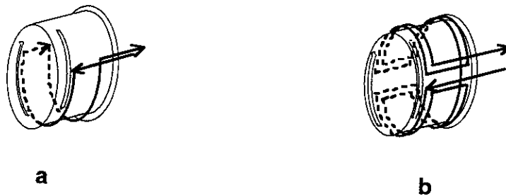
FIG. 4: The shape of the NMR coils for the NH 3 target and ND 3 target.
