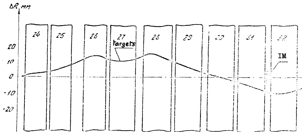
Fig. 3. Section of the disturbed orbit. IM = pulsed magnet.
