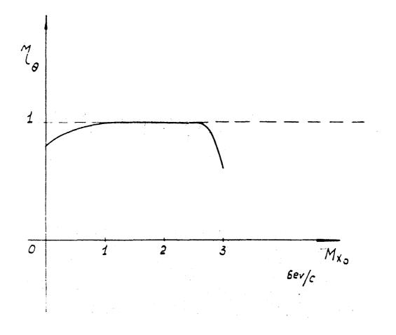
Fig. 3. Geometrical efficiency in terms of the angle of the neutron spectrometer against the missing mass  $M_{\mathbf{x}}$ .
