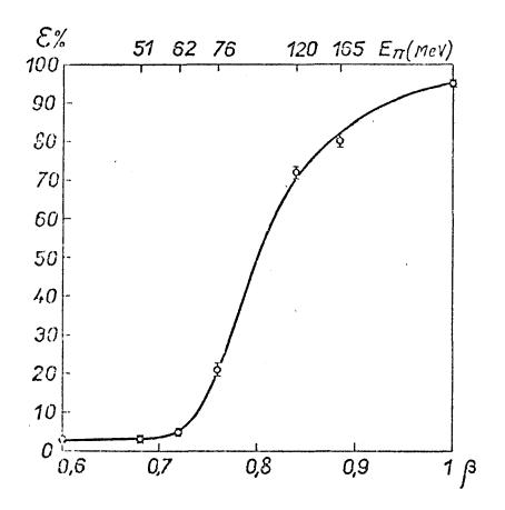
Dependence of Čerenkov counter's efficiency  $\mathcal{E}$  on the velocity  $\mathcal{A}$ and kinetic energy  $\mathbb{E}_{\mathcal{T}}$  of the  $\gamma$  mesons. The curve is drawn by hand from the experimental data.
