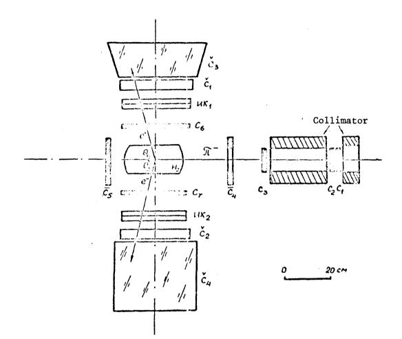
Diagram of experimental device.  $\gamma$  beam incident on hydrogen target H<sub>2</sub>, C<sub>1</sub> - C<sub>2</sub> - scintillation counters, Č<sub>1</sub> and Č<sub>2</sub> - threshold Čerenkov counters, Č<sub>3</sub> and Č<sub>4</sub> - Čerenkov spectFometers, IK, and IK<sub>2</sub> - spark chambers.
