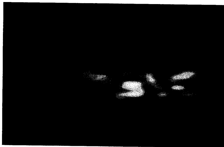
Figure 5. Far-field intensity distribution of the frequency doubled beam obtained at an incident fluence onto the crystal of 200 \text{ GWcm}^{-2} .
