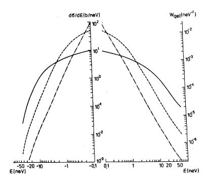
Fig. 2 Differential cross-section  $d\sigma/d\epsilon$  (b/neV) and relative probability  $w_{qel}$  (neV<sup>-1</sup>) of UCN quasielastic scattering due to diffusive motion of hydrogen atoms for different values of the diffusion coefficient D: solid line -  $D=1.85\cdot 10^{-5} {\rm cm}^2/{\rm s}$ ; dashed line -  $D=1.85\cdot 10^{-6} {\rm cm}^2/{\rm s}$ ; dashed-dotted line -  $D=1.85\cdot 10^{-7} {\rm cm}^2/{\rm s}$ . Incident neutron energy 50 neV.
