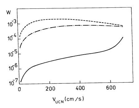
Fig. 1 Calculated UCN loss coefficient as a function of the normal to the surface component of neutron velocity for a beryllium wall covered with water layer of different thickness: solid line - clean beryllium, dashed-dotted line - 100 Å, dashed line - 200 Å.
