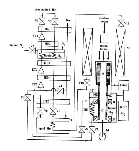
Fig.1. Schematics of the liquefier-refrigerator and the cryogenic reactor
