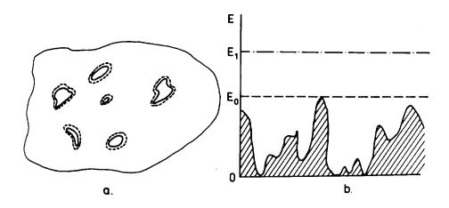
Fig.1 a. The UCN with energies below the boundary energy  $E_0$  must be trapped according [19] into micropores by tunneling from thin layers (thickness  $\sim \lambda \sim 100$  Å) surrounding the pore.
