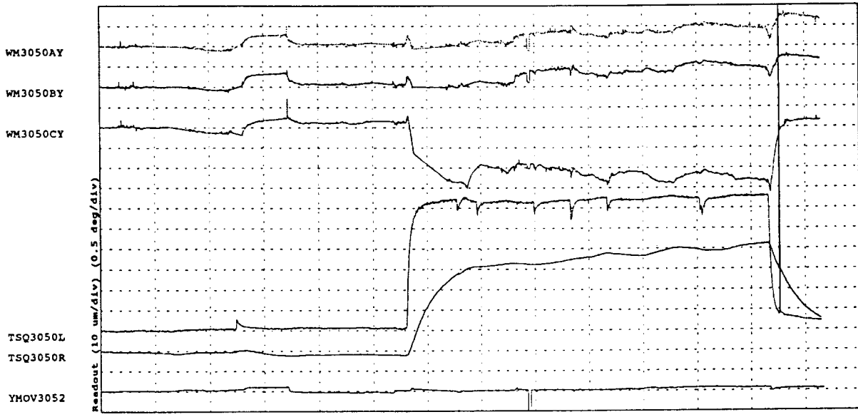
Fig. 9 Same as Fig. 8 but with correction of the wire readings for the motion of WT3, the LVDT reading of the mover system and temperature effects.
