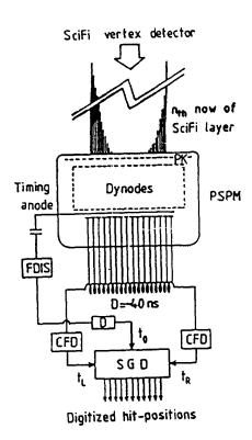
Fig. 1. Conceptual design of the topologies trigger device; a) Mechanical structure, b) Associated electronics.
