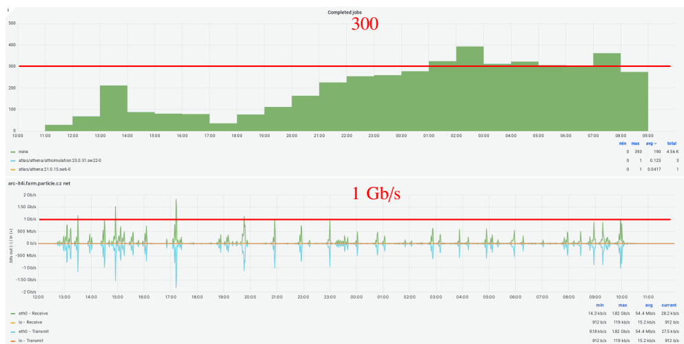
Figure 6. The atlas-cvmfsexec usage. The upper plot shows number of completed jobs in 1 hour bins. The lower plot shows network traffic at the same time period.
