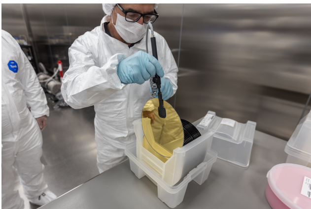
Fig. 3 Wafer cassette containing one production Lot (25 wafers). The wafer's gold backside is visible.
