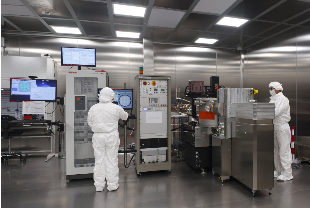
Fig. 5 Form Factor PAC-200 probe system + S500 Parametric Keithley tester used to characterize the response of the FBK NUV-HD Cryo SiPMs. The entire system is located in a new ISO-6 353 m 2 clean room packaging facility called the Nuova Officina Assergi (NOA) constructed at the Istituto Nazionale di Fisica Nucleare (INFN) Laboratori Nazionali del Gran Sasso (LNGS).
