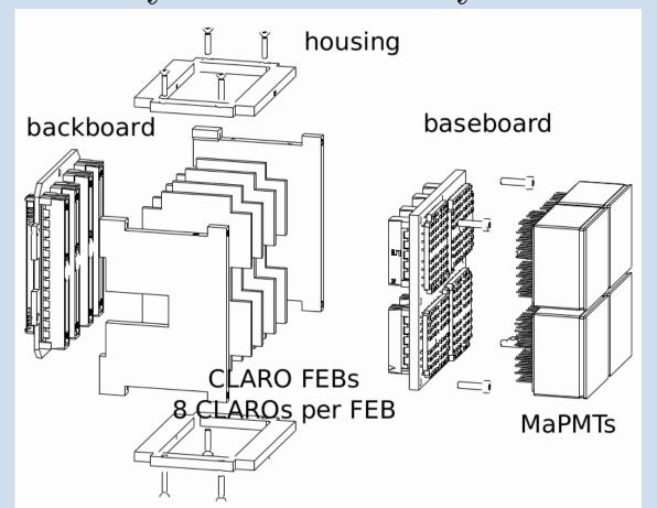
The Photon Detector Module (PDM) is the smallest logical unit allowing the interface of the RICH components with the upgraded LHCb readout architecture through the GBT
