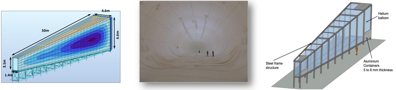
Figure 1: (Left) The steel decay vessel considered for the SHiP comprehensive design study; (centre) a photo of the kind of large helium bag envisaged; (right) the aluminium frames envisaged to hold the bag in place.
