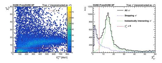
**Figure 5**: The  $\chi^2_{\pi^{\pm}}$  distributions of charged pions are shown. Left plot shows a two dimensional distribution as a function of truth  $E_K$ . Right plot shows one dimensional distribution of  $\chi^2_{\pi^{\pm}}$ . Reconstructed charged pions which are matched with truth-level charged pions are used in this plot.
