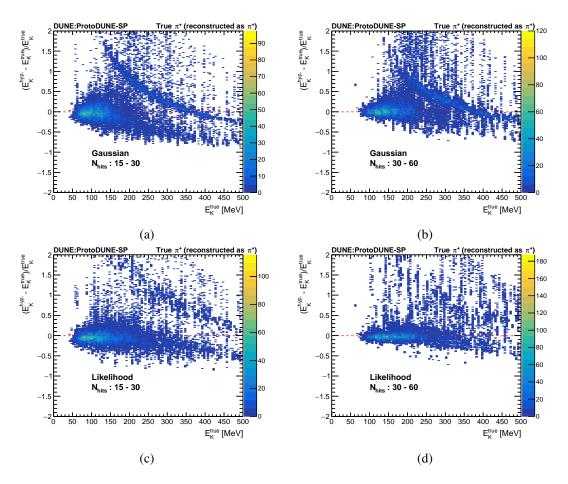
**Figure 8**: Example two-dimensional distributions of the fractional energy residual from the Gaussian approximation method (top) and the maximum-likelihood method (bottom), using 15 to 30 (left) and 30 to 60 (right) hits.
