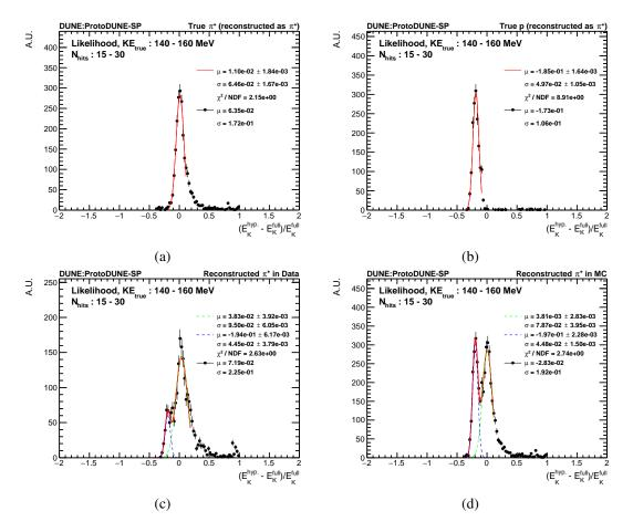
**Figure 13**: Example distributions of the fractional energy residual using range-based  $E_K$  as reference. Results come from reconstructed charged pions with 15 to 30 hits. Top plots show results for MC true pions (a) and true protons (b). Bottom plots show results using all reconstructed charged pions for data (c) and the MC sample (d), where green and blue Gaussian functions represent charged pion and proton contributions, respectively.
