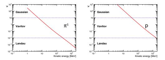
**Figure 2**: Three regions are defined using the  $\kappa$  value. If  $\kappa > 10$ , the Gaussian PDF is used. If  $\kappa < 0.01$ , the Landau PDF is used. Otherwise, the Vavilov PDF is used. Plots are drawn for charged pions (left) and protons (right) in LAr using typical pitch (0.65 cm) of the ProtoDUNE-SP.
