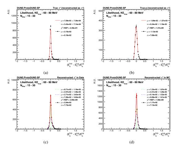
**Figure 12**: Example distributions of the fractional energy residual using range-based  $E_K$  as reference. Results are coming from reconstructed charged pions with 15 to 30 hits. Top plots show results for MC true pions (a) and true protons (b). Bottom plots show results using all reconstructed charged pions for data (c) and MC sample (d), where green and blue Gaussian functions represent charged pion and proton contributions, respectively.
