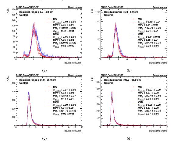
**Figure 16**: The dE/dx of beam muons is shown as a function of residual range for both data (blue) and MC (red). The results of fits to a Landau function convoluted with a Gaussian are also shown in the legends. The  $\sigma_{\text{Landau}}$  is intrinsic width of the Landau function, MPV is fitted most probable value, Par<sub>2</sub> is normalization factor, and  $\sigma_{\text{Gaus}}$  is the width of the Gaussian.
