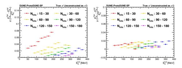
Figure 14: Summarized plots of energy measurement performance of the hypothetical track-length fitting method based on the maximum-likelihood method. Resolutions (left) and fractional biases (right) are shown as functions of charged pions' range-based  $E_K$  and number of hits. Pure secondary charged pions are selected from the MC sample.
