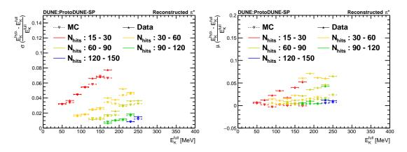
Figure 15: Summarized plots of energy measurement performance of the hypothetical track-length fitting method based on maximum-likelihood method. Resolutions (left) and fractional biases (right) are shown as functions of charged pions' range-based  $E_K$  and number of hits. All reconstructed secondary charged pions passing the stopping charged pion cut are used. Monte Carlo points are shown with dashed horizontal bars and the data points are shown with solid horizontal bars.
