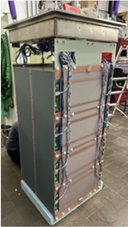
Figure 17: Left: A photograph of one of the four ton-scale LArTPC modules for the 2x2 Demonstrator, a prototype of the DUNE ND. Right: an example cosmic ray imaged in true 3D using a 102,400-channel LArPix-v2 system in this module (right).
