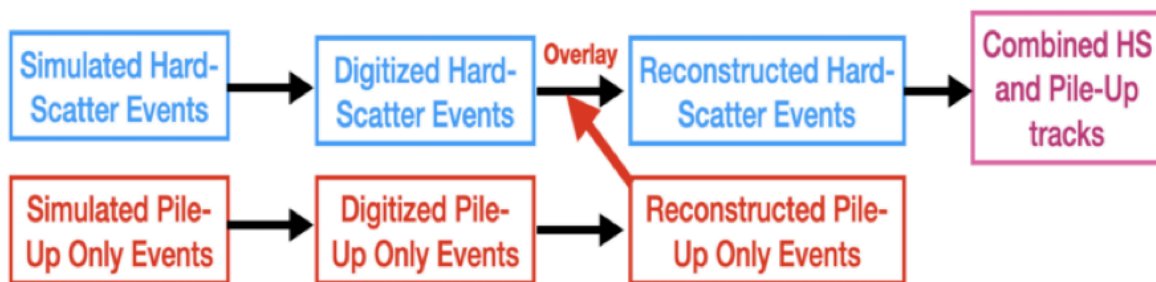
Figure 2. In the track overlay method, pre-reconstructed pile-up tracks are overlaid onto HS digitized events, followed by the reconstruction process.
