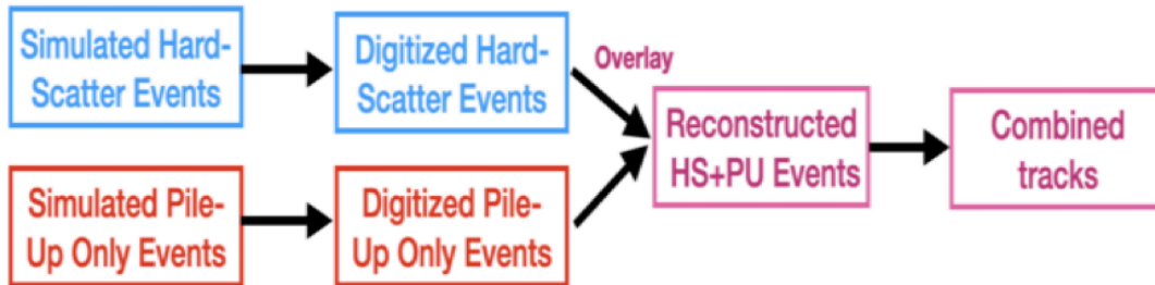
Figure 1. Diagram of the MC overlay process, where simulated pile-up collisions are digitized separately and then combined, followed by the reconstruction algorithm.
