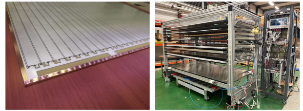
Figure 3: Left: A BIL readout panel, with copper tape end matching resistors in evidence. Right: Cosmic rays test stand.
