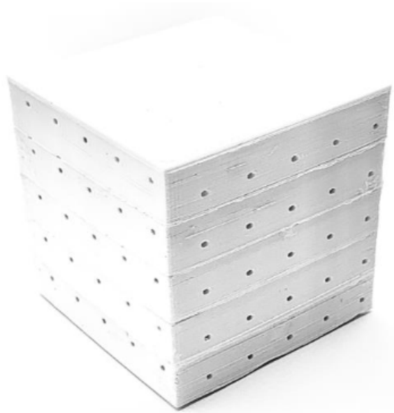
FIG. 3. Left: SuperCube illuminated with UV light prior to completion. The absence of a white reflector layer on the SuperCube’s top surface provides a clear view of the inner structure, featuring optically isolated PS cubes intersected by WLS fibers. Right: FIM manufactured 5x5x5 SuperCube, requiring no post-processing.
