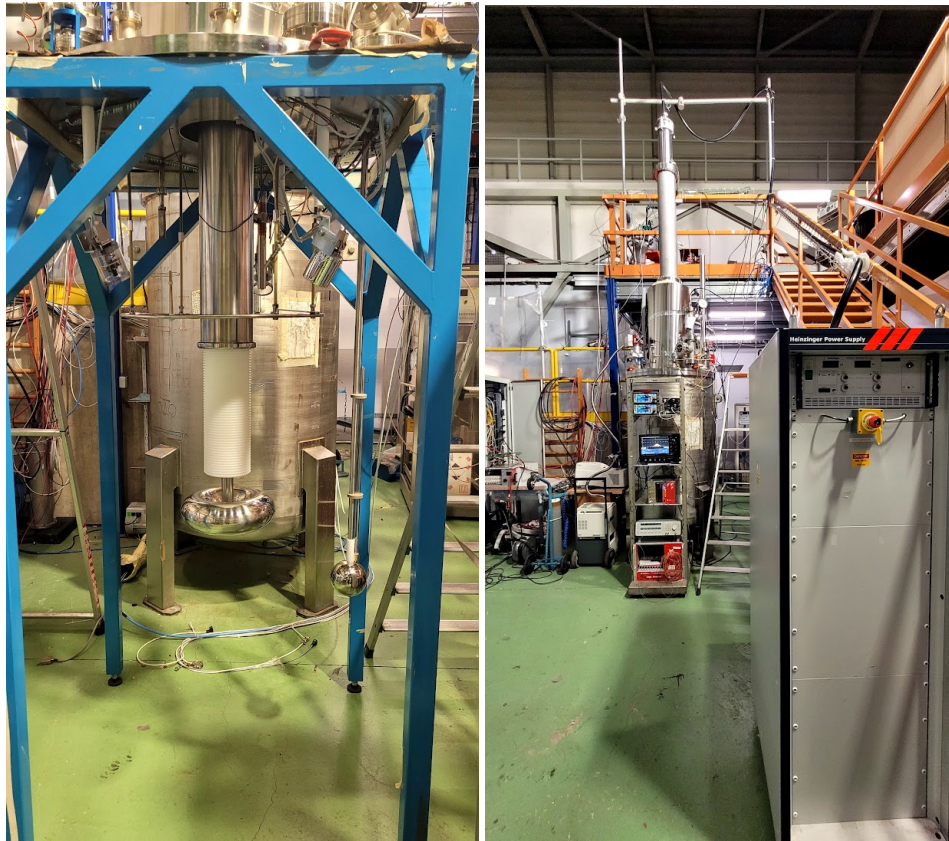
Figure 16: Left: the new 300 kV HV feedthrough for NP02 being tested in standalone mode. Right: the test stand of the HV feedthrough for long term stability validation.
