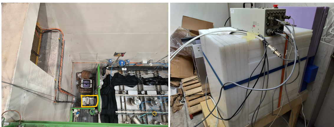
Figure 10: PNS installation in VD Cold Box, Left: Yellow marker indicates the location of the PNS as seen from the top, Right: Polyethylene shielding covering the DDG.
