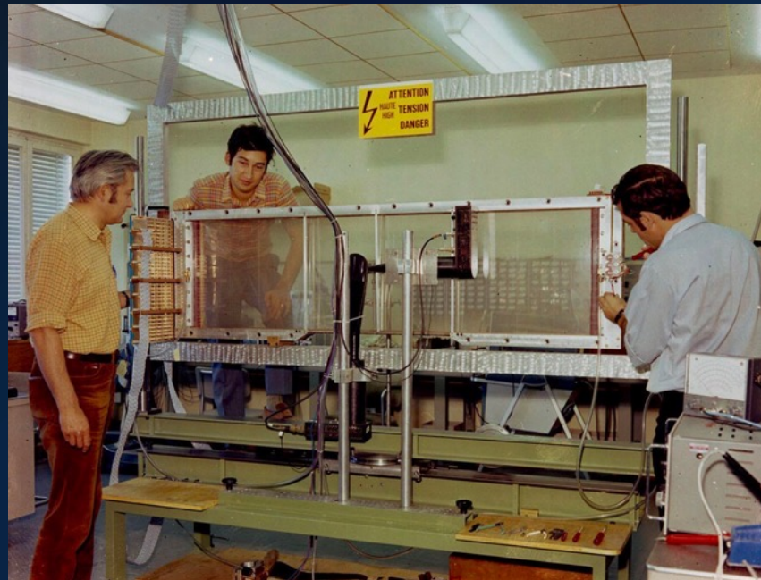
1971-1972 – Large-size Multiwire Proportional Chamber
