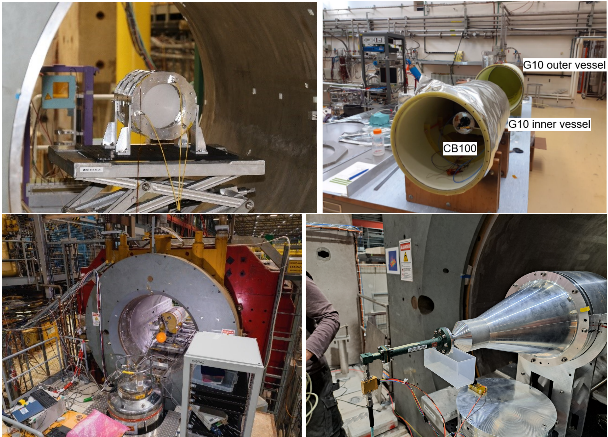
Figure 3: Pictures of MADMAX prototypes: OB200 in the Morpurgo magnet (top left) CB100 inside the G10 cryostat (top right) and inside the the Morpurgo magnet (bottom left), CB200 inside the Morpurgo magnet (bottom right).
