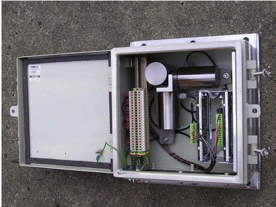
Figure 6.10: Sensonics model SA-3 safety seismic switch
