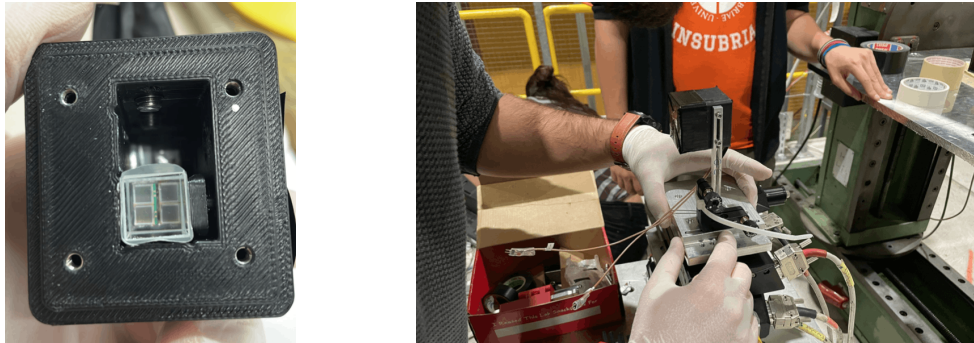
Figure 78: Left: Single crystal read out with 2 \times 2 matrix of four 4 \times 4 \text{ mm}^2 SiPMs. Right: Installation of crystal on H2 beam line during fall 2022 test beam.
