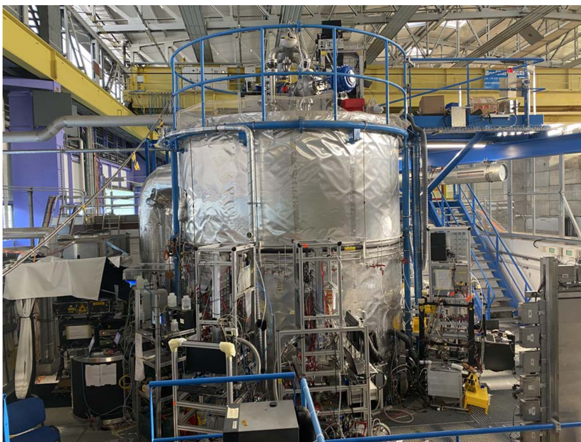
Fig. 4: CLOUD15 run (19 Sep - 22 Nov 2022). CLOUD and some of its analysing instruments in the T11 experimental zone during the CLOUD15 run. During operation, the T11 beam emerges from the lower right hand side of the figure and passes through two counter planes (B and VH; the latter is seen at the right hand edge of the image) before crossing the CLOUD chamber located inside a thermal housing. Mass spectrometers and other instruments mounted on the platform continuously extract air from the CLOUD chamber via sampling probes to analyse its contents. FLOTUS is located on the opposite side of CLOUD and is not visible in the image.
