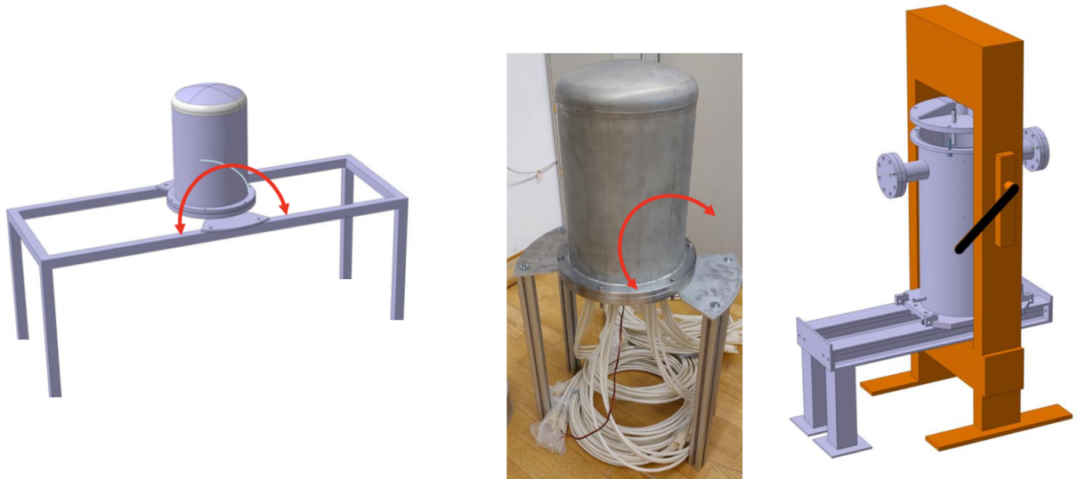
Figure 25: Conceptual design of the support stand for the fixation of the mechanical vessel and the installation of the boards and cables inside (left), photo of the simple support used for testing the assembly steps (middle) and conceptual model of the pressurized tank (right).
