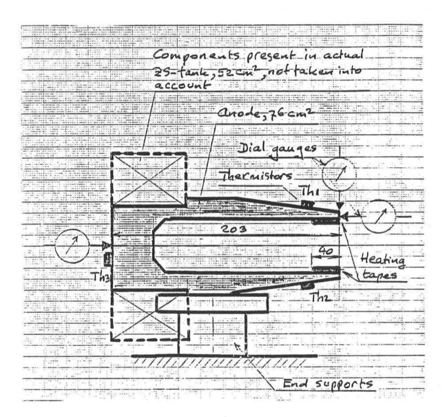
Fig. 3 -Measurement of the Thermal Deformation of the Anode
