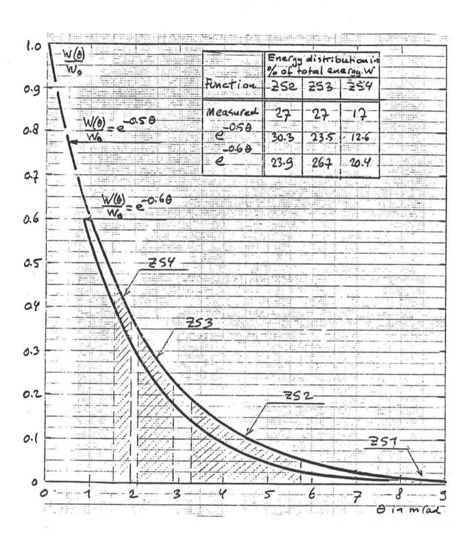
Fig. 2 - The Angular Secondaries Energy Distribution emerging from the
