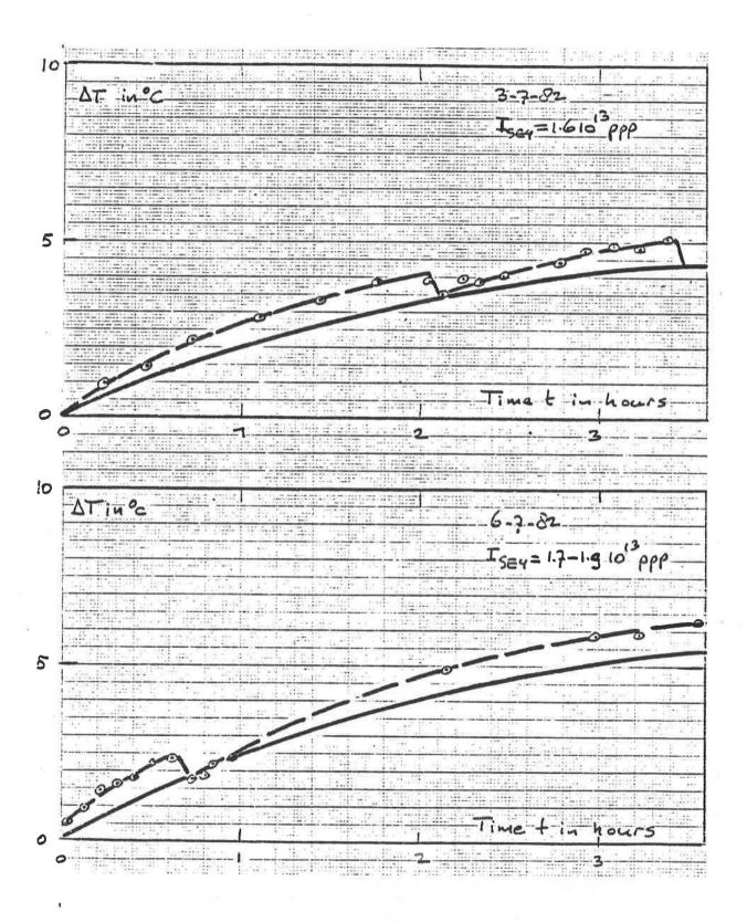
Fig. 1 - Temperatures of the ZST-anode, Slow Extraction in LSS2
