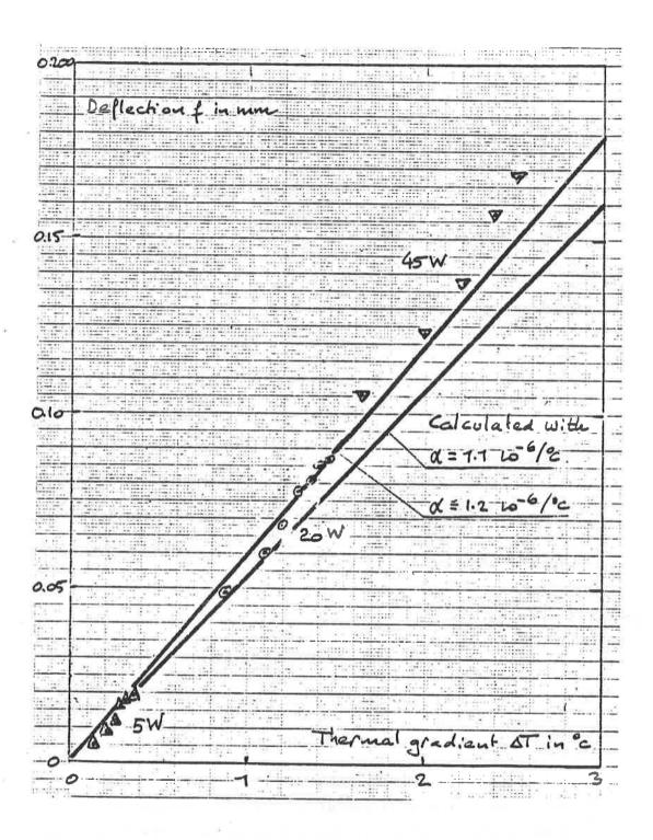
Fig. 4 - Deformation of the Anode as a Function of the Thermal Gradient
