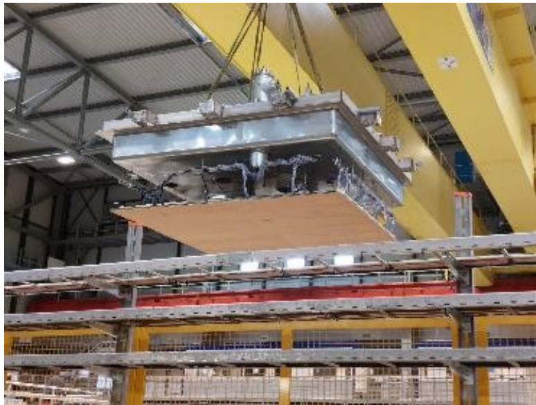
Figure 8: CRP2 suspended from the cold-box roof being moved from the Faraday cage to the cold-box location
