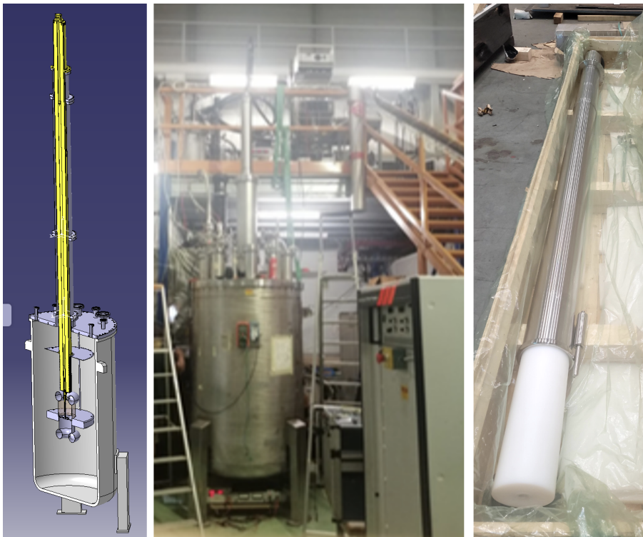
Figure 24: Testing station (left and center) for the newly built HV feed-through (right).
