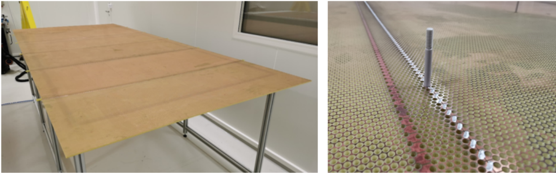
Figure 1: Left: Photo of one anode panel after gluing; Right: a closeup view of the induction layer with the glued junction and silver printed pads
