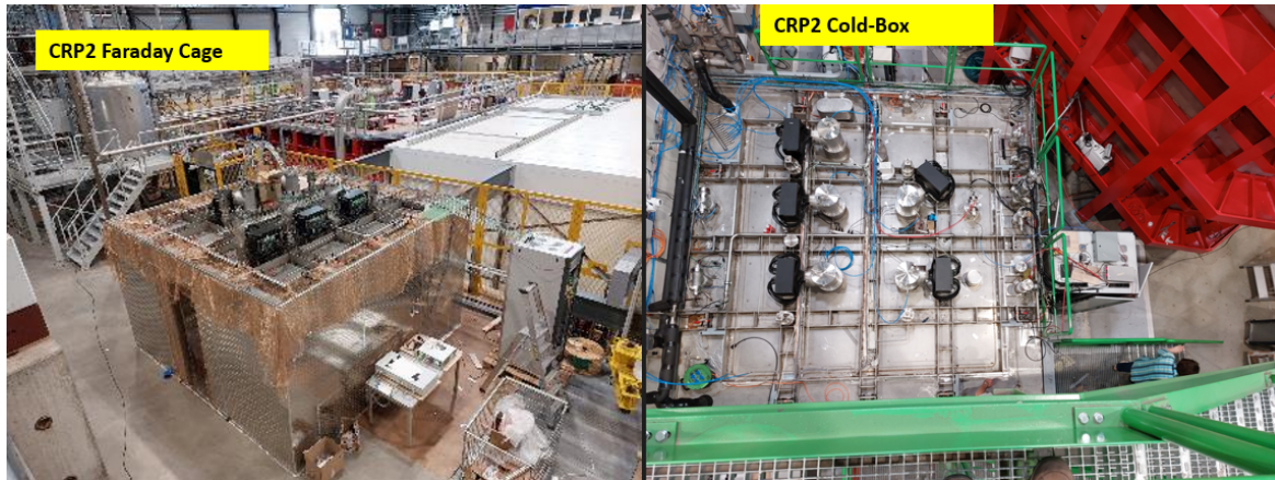
Figure 10: Top drift readout chain installed in the Faraday Cage and cold-box setups for the tests of CRP2 in July 2022
