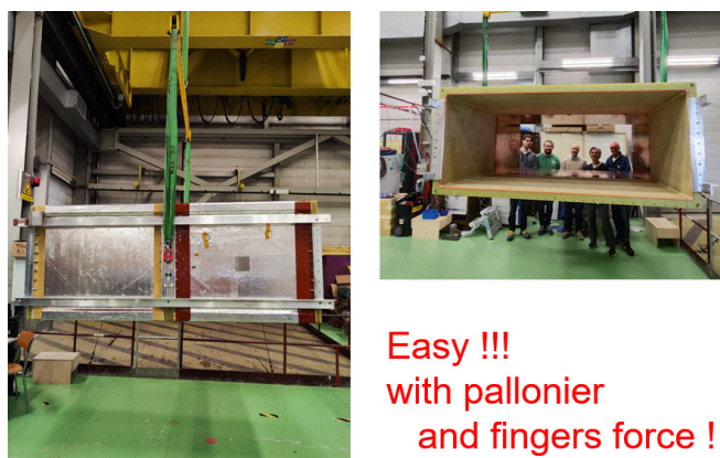
Figure 15: Assembling FC0 and FC1 into a "full" scale HATPC
