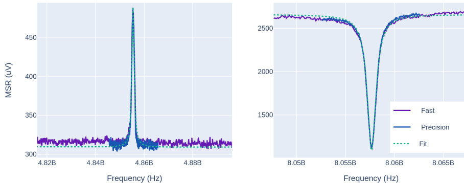
Figure 3. Example of two calibration experiments executed using Qibocal on quantum processors. On the left a qubit spectroscopy and on the right a resonator spectroscopy for a qubit hosted at Quantum Reasearch Center (QRC) in Technology Innovation Institute (TII).
