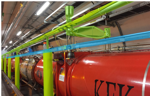
Figure 4: Photo of the low-beta magnets before the physic detector. The alignment systems are highlighted: Hydrostatic Levelling System with water network, support pillars and sensors (light green) and the Wire Positioning System with sensors, stretched wire, wire protection system (light blue).
