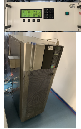
(b) Chiller and controller: Huber Unistat 380
