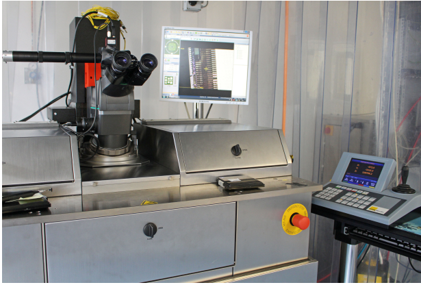
(a) Probe station: Süss PA300
