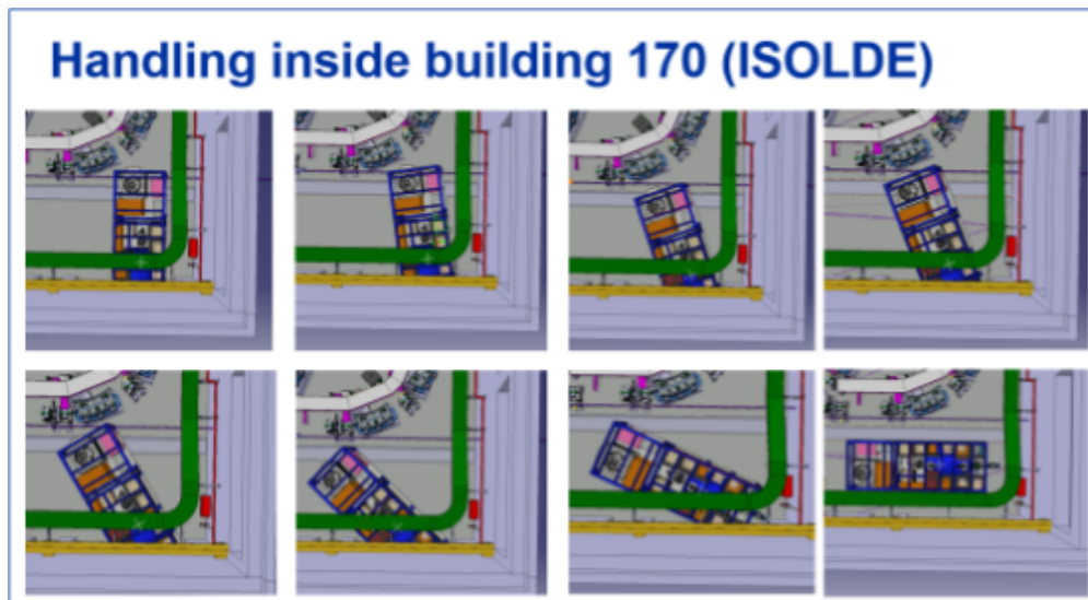
Figure 33: Handling sequence defined using 3D integration model.
