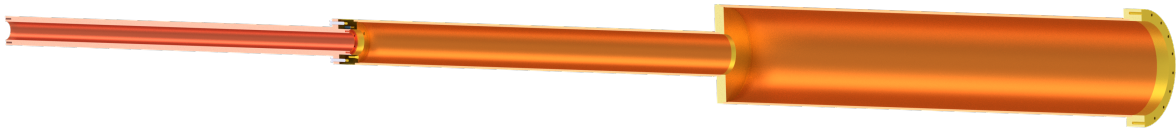
Figure 15: Rendered 3D model of the 4K cryostat main chamber. The model has been approved by the CERN mechanical workshop and is currently manufactured.
