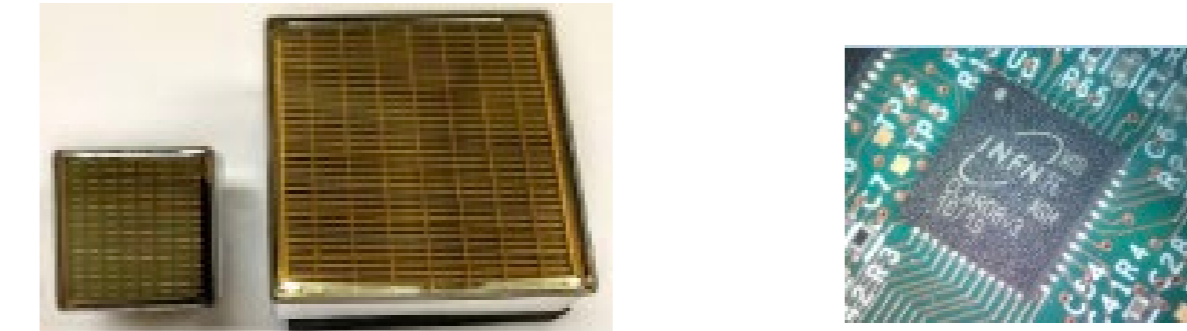
Figure 4: Left: Hamamatsu MaPMTs the R11265 (R-Type) on the left and R12699 (H-Type) on the right. Right: CLARO ASICs.
