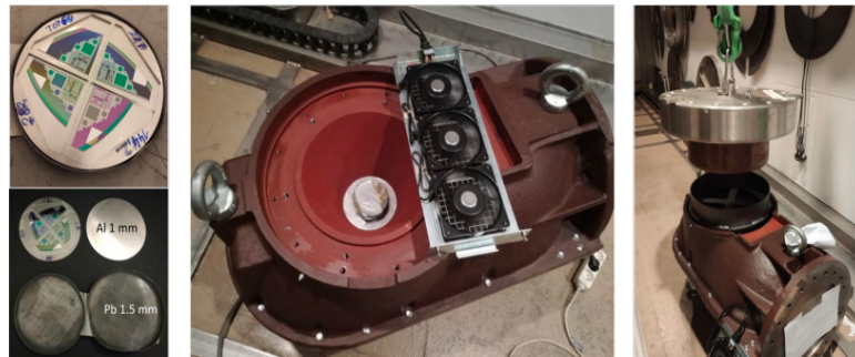
Figure 2. The sample holder for the ^{60}\text{Co} irradiation at UJP Praha, made with material thickness of 1.5 mm Pb and 1 mm Al to minimise the dose induced from scattered low energy charged particles and to achieve Charge Particle Equilibrium according to Total Ionising Dose Irradiation Standards [4].
