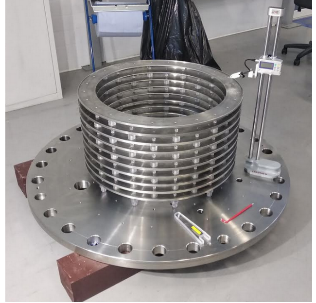
Fig. 33: Left panel: sketch of the Zeolite-based purification unit. Right panel: sample of preliminary assembling of the inner structure.
