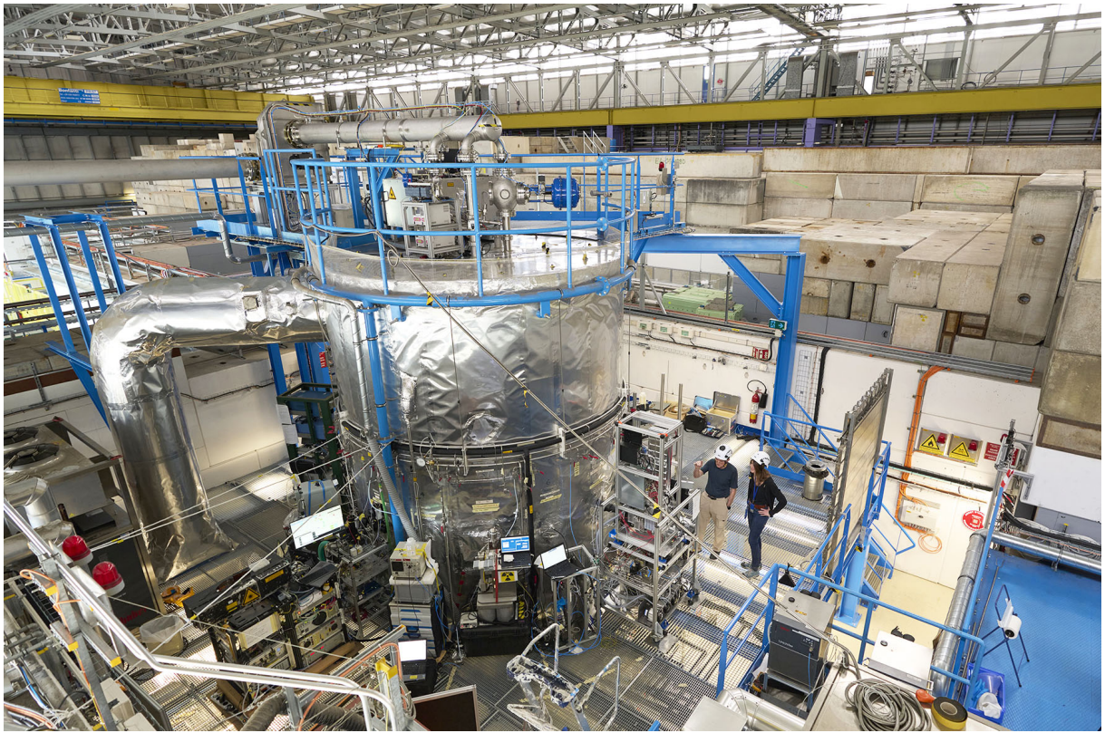
Fig. 6: CLOUD15T run (23 Mar - 2 May 2022). CLOUD and its analysing instruments in the T11 experimental zone during the CLOUD15T technical run to re-commission CLOUD following the rebuild of the T11 beamline, the CLOUD facility and its infrastructure during LS2. During operation, the T11 beam emerges from the concrete shielding blocks on the right hand side of the figure and passes through two counter planes (B and VH; the latter is seen mounted on the edge of the platform) before crossing the CLOUD chamber located inside a thermal housing. Mass spectrometers and other instruments mounted on the platform continuously extract air from the CLOUD chamber via sampling probes to analyse its contents. The HORUS instrument is in the left foreground.
