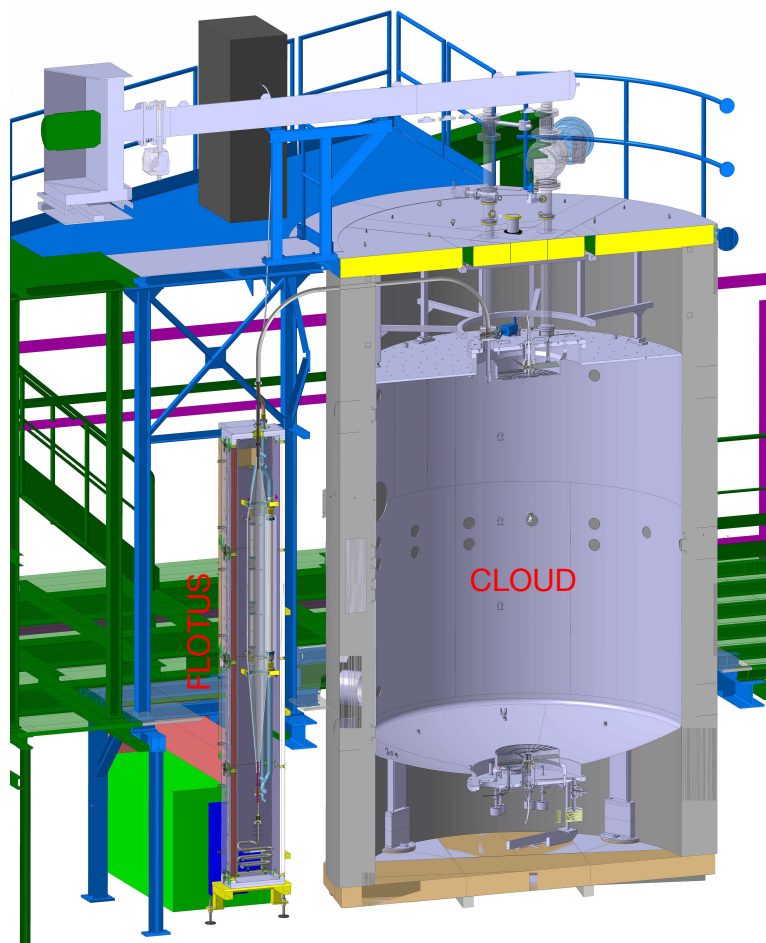
Fig. 9: FLOTUS (FLOW TUBE System) at CLOUD. FLOTUS is a 3 m laminar-flow quartz drift tube in which organic and other vapours receive hydroxyl radical exposures corresponding to several days in the real atmosphere. The outflow from FLOTUS is directed into the CLOUD chamber for studies with “aged” organics. All the operating conditions of FLOTUS (gases, UV irradiation, relative humidity and temperature) are controlled independently of the CLOUD chamber.
