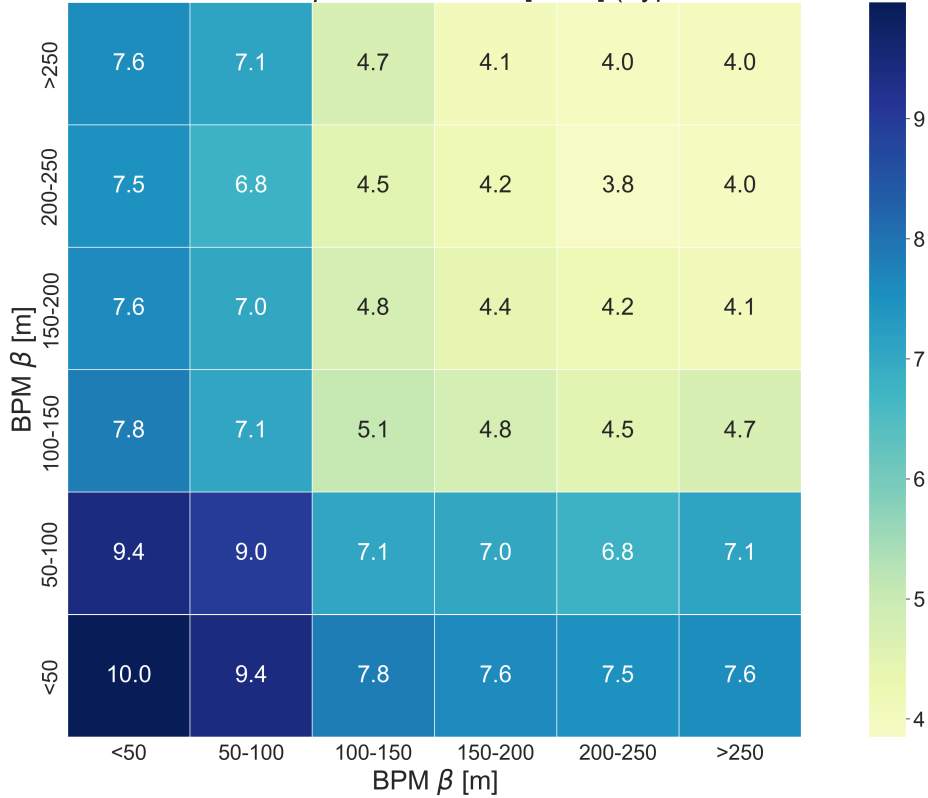
Figure 17: Computed standard deviation (in mrad) on phase measurement between standard BPMs for the LHC Run 2 (2018, \beta^* = 30 cm) for different \beta -functions combinations of BPMs.
